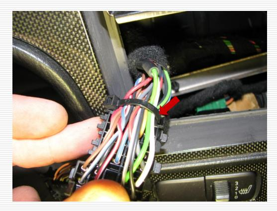
Splay the wires so that the upper portion of the connector is separated.
