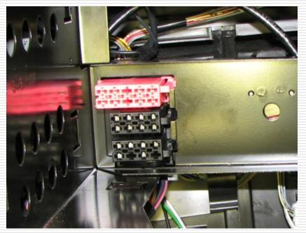
Test the retention of the connectors by pushing on them gently. They should not move.
