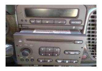
Step 4: Remove the ac-panel by gently pulling it loose with a screwdriver.
