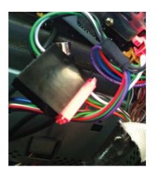
Step 9: Now the device needs to be energized, this is done through the brakeout adapter for the 12 volt outlet included in the kit. By putting adaptor between the cigarette lighter socket and its connectors.
